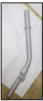
**22.** Take our short shifter kit PR98016P and use actuator part (marked with red) and glue it together with the upper part, using quality 2K-metal epoxy adhesive:
