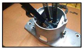
32. Insert buffer plate, install carrier plate (some preassure is needed to press down the carrier plate – use distance blocks to clear gearshift lever lower part) following washers and nuts installation:
