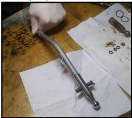
NOTE: If gearshift lever was glass blasted - mask the shifter actuator and paint the upper part of the gearshift lever:
