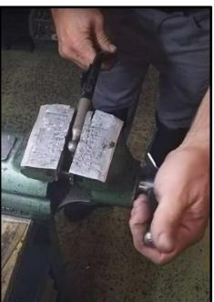
19. While heating the gearshift lever, move upper part in left and right direction while
