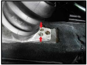
**8.** You can now remove complete gearshift lever unit. Usually ball cup bushing will stay on the shifter lever actuator. You can either remove it and set it aside or put it back in the ball cup bushing cylindrical base as shown on the picture:
