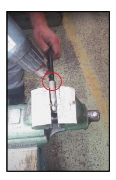
20. You will end up with two parts upper and lower (actuator) part of gearshift lever.
