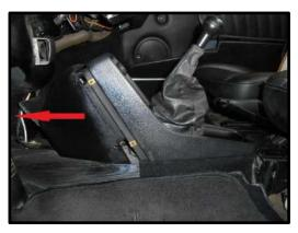
**3.** Remove three ground screws holding the center console. Two screws are in the front part of the console:
